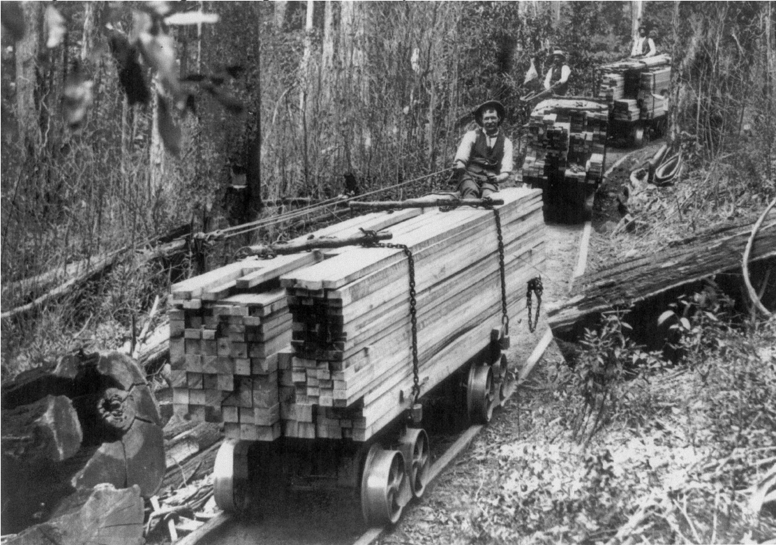
With a firm grip on the brake ropes the brakemen hold their loads steady for the photographer somewhere below "The Take-off" on the Mississippi tramway.
